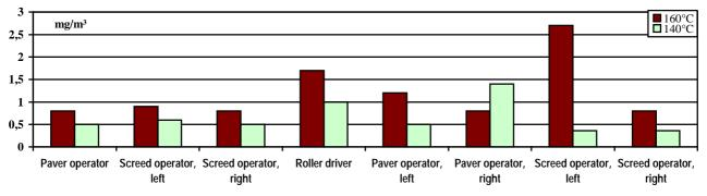
Figure 4: Comparison of exposure to fumes and aerosols from bitumen by laying normal and low temperature asphalt at a construction site in France
