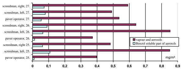
Figure 2: Measurements comparing the United States (benzol soluble part of aerosols) and the German procedure (fumes and aerosols) (asphalt temperature 160°C; Shell, 1999)
