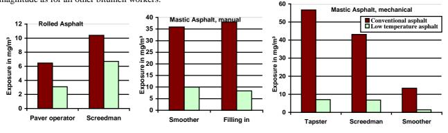
Figure 3: Exposure to fumes and aerosols from bitumen by laying normal and low temperature asphalt
