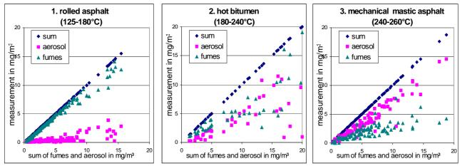
**Figure 1:** Comparison of the proportions of fumes and aerosol concentrations from hot bitumen. 1. Working with rolled asphalt in road paving. 2. Working with hot bitumen in pouring process. 3. Mechanical working with mastic asphalt in road paving. The diagram shows only values up to 20 mg/m<sup>3</sup> in the cited working temperature range.
